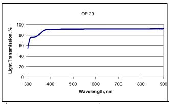
Measured at 0.03 mm [0.001in] per DSTM-501<sup>‡</sup>
