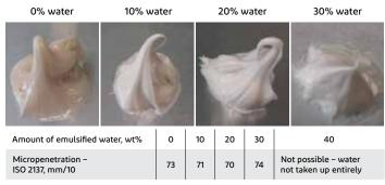
Able to absorb up to 30 wt% of water without loss of consistency
